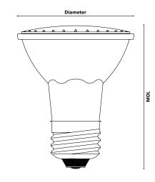
MOL : 3 <sup>1</sup>/<sub>8</sub> in. (79 mm) Dia. : 2 <sup>1</sup>/<sub>2</sub> in. (63 mm)
